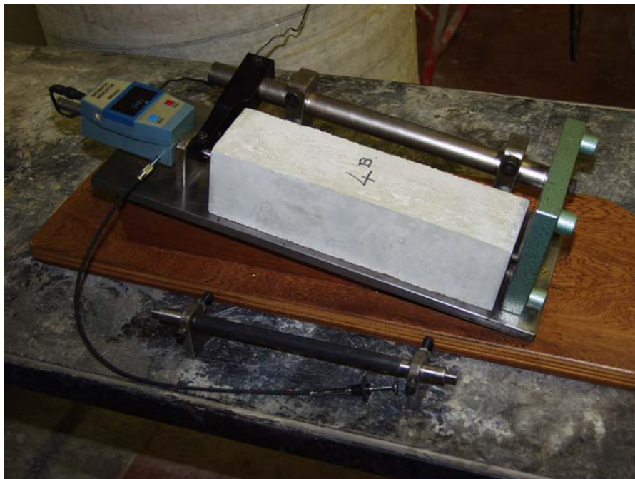
Figure 3: Shrinkage measurements using standard comparator (accuracy 0.001 mm)
