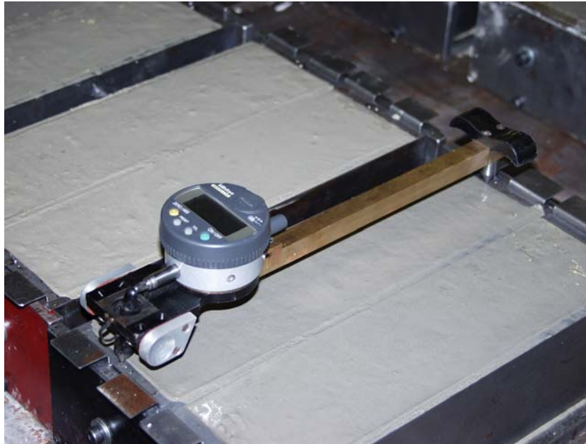
Figure 2: Shrinkage measurement using DEMAG gauge (0.001 mm accuracy) between 0 and 1-day
